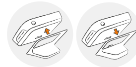
Attaching the B.Box Evo Stand or the B.Box Evo Battery Stand
